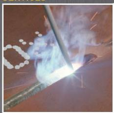
Welding Hardox requires low preheating thanks to the low carbon equivalent. The plate flatness and narrow tolerances facillatetes automatic welding and shortens preparation time for fit up and tracking. You also get very good HAZ properties due to the high toughness and low levels of steel impurites.
