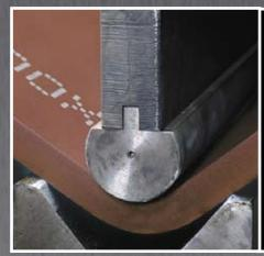
Bending The steel quality and surface finish make a tight bending radius possible, especially when bending thinner plates. The consistent properties and the close thickness tolerances ensure very high precision bending results.
